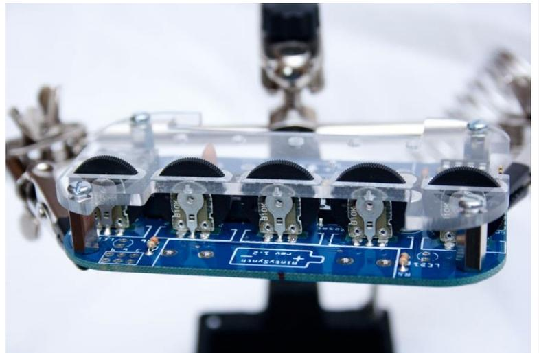
Now you can remove the bottom four screws and the acrylic cover, and we'll add the final few components. Install the two LEDs as shown, with the red one on the left. The LEDs have a small flat on the negative side of the housing (this is also the side with the shorter wire lead). **This side needs to point toward the thumbwheels. The negative lead will go through the round pad.** You can bend the leads outward slightly like you did with the resistors to help hold them in place while you solder.
