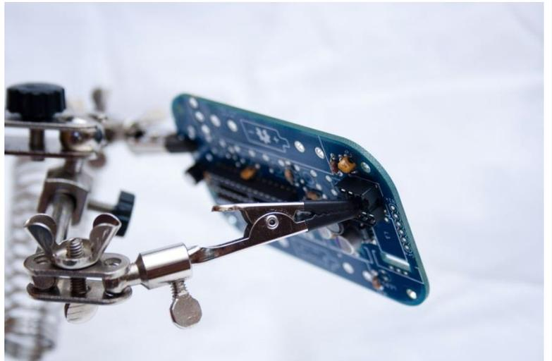
As previously, clip the pins close on the back after soldering. The larger socket (for the AtMega IC) is shown here, with the pins clipped.
