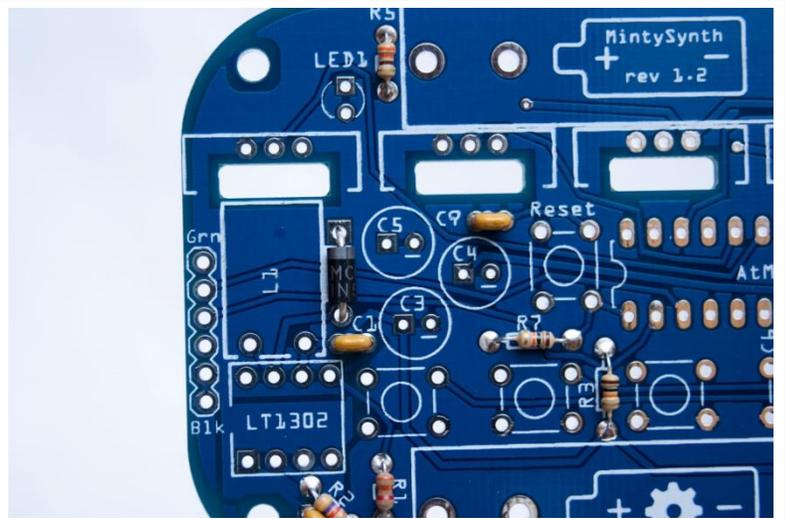
Next is the reset button. Note the direction of the legs; on this button they point toward the top and bottom edges of the PCB. The buttons require a small amount of force to snap them in place. It works well to push them down evenly with one fingernail on each side of the button. The button should seat fully onto the PCB and hold itself in place while you solder it.
