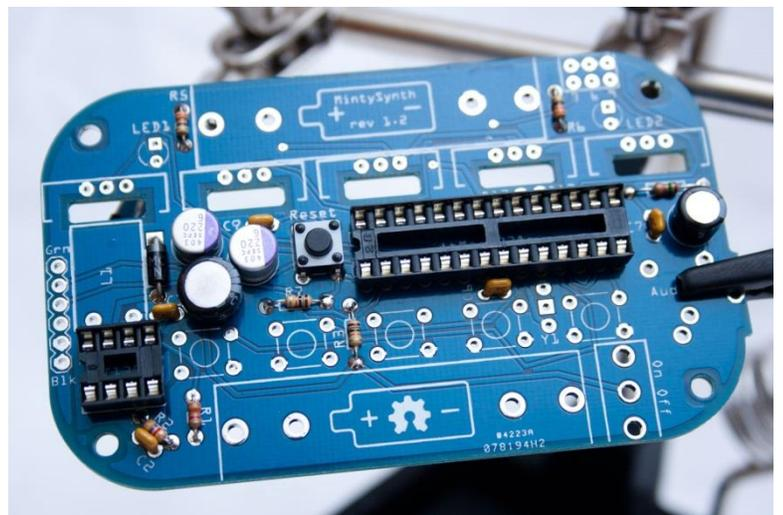
Here one clip on the helping hand is being used to hold the smaller socket in position for soldering. It's a good idea to solder one pin on the socket, then check to make sure it is still fully seated, solder another pin at an opposite corner, make one last check, and finally solder the remaining pins.
