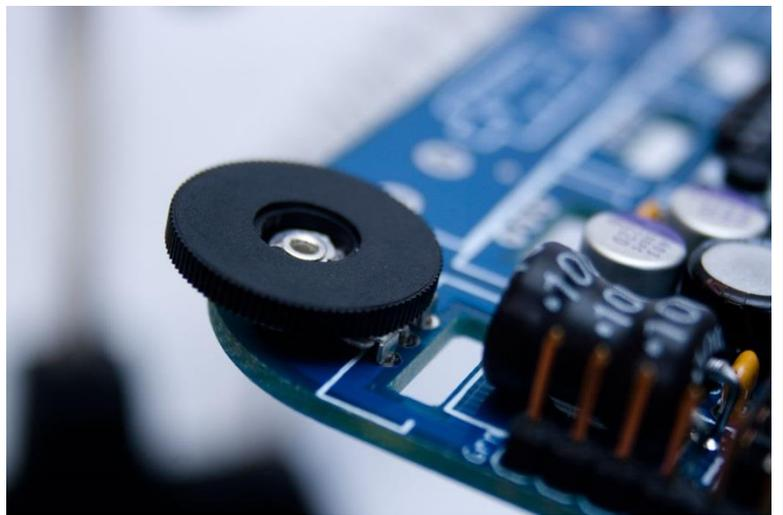
Then, keeping the pins fully seated, gently fold the thumbwheel upward until it is vertical, bending the pins as close to their shoulders as possible.
