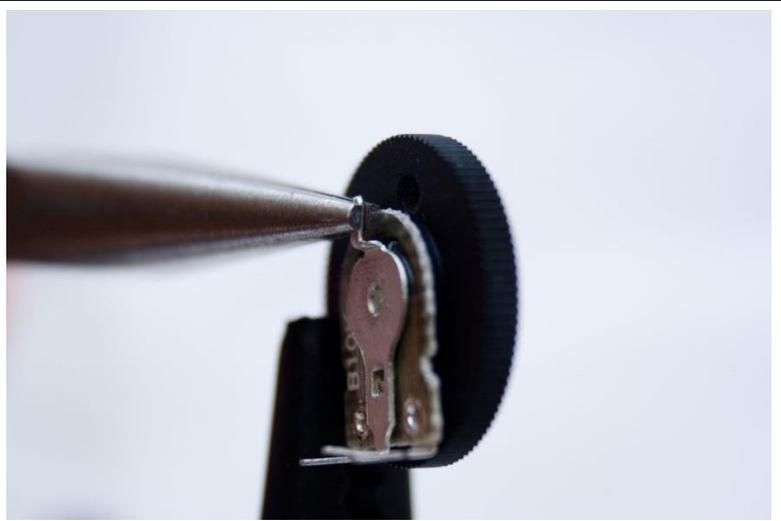
Now, use your cutters to clip the pin so it is about 1mm long (past the shoulder) as shown. Repeat this process for all five thumbwheels. Test the fit of the pins in the underside of the acrylic—each pin should slip into the small hole, pulling the thumbwheel snug against the side of its slot. If a pin won't reach the hole, you can bend it out away from the wheel a little more until it fits.
