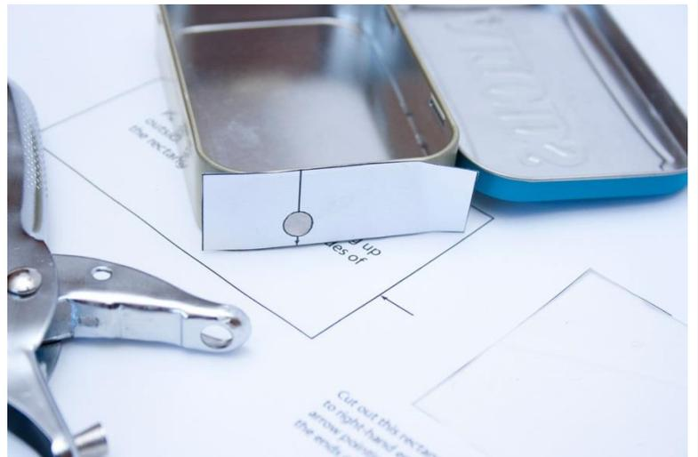
Next, cut out the rectangle on the lower half of the page and glue it onto a sheet of thin cardboard (cereal-box cardboard, etc.). Then cut it out on the outline. The cardboard will serve to insulate the bottom of the PCB from the tin.
