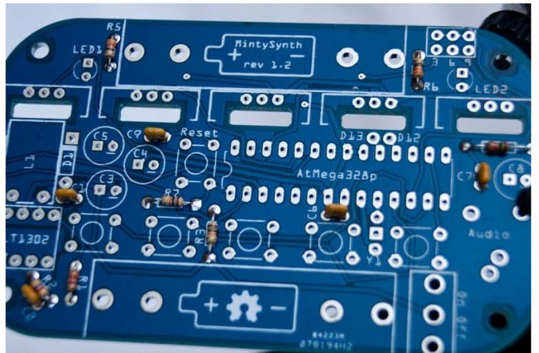
Next we'll install the diode D1, which is used by the boost circuit. It is polarized, so be sure that the end with the grey band is pointed up, as shown. Install it just as you would a resistor.
