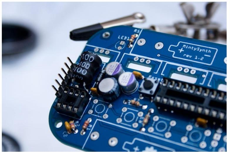
Now we're ready for the five tall buttons. It should be clear from the PCB, but note that these are oriented in the opposite direction of the reset button that we installed earlier (the legs are towards the left and right sides of the PCB). Again, you snap them into place by putting even pressure on both sides of the housing. Be sure that each is fully seated before soldering.
