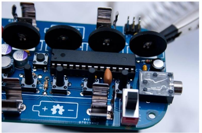
If you'll be using the preinstalled software, put the jumper in place in position 3 as shown. You also have the option of using digital pin 6 or 9 as the audio output if you're using other software. **Note: don't forget the jumper, or you won't get any sound. It's easy to forget.**
