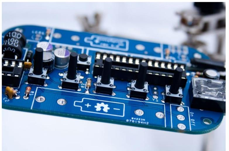
Next is the ceramic resonator, Y1. There's no polarity, so either way is fine. Again, the second clip on the helping hand is useful here to hold it in place while you solder. Check after soldering one pin that it is seated vertically.
