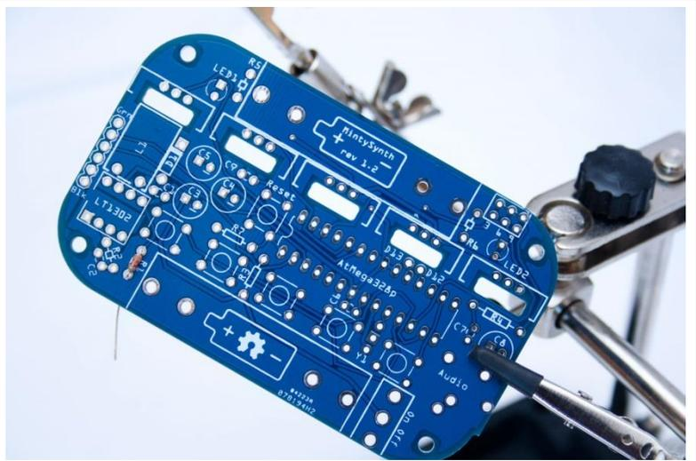
We'll begin with resistor R1 (3.3 k $\Omega$ ). Form the resistor into a staple shape and insert it. Resistors are not polarized, so it doesn't matter which way it goes. Try to be sure to seat it all the way into the PCB.
