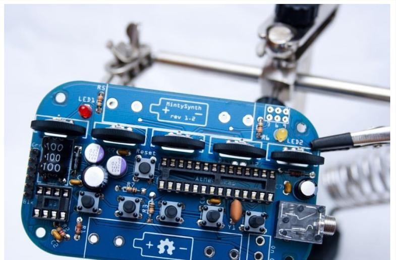
Next is the header for the jumper, as shown. Install it like you did the FTDI header, with the short ends of the pins through the PCB.
