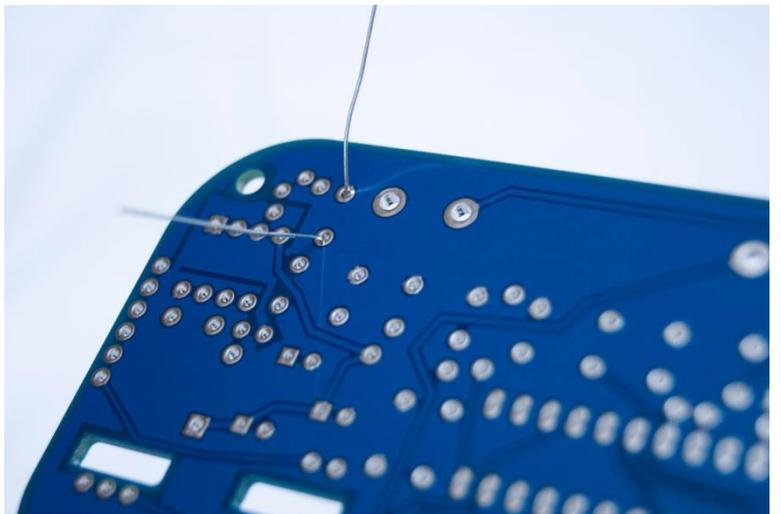
Next you can solder the rest of the resistors in place, checking the parts list to make sure you have the correct value for each. Here they are before clipping the leads.
