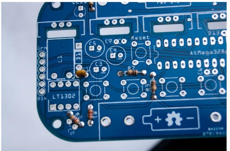
Here all the ceramic capacitors are in place. Again, clip the leads short on the bottom.
