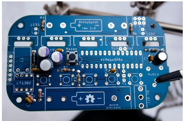
Next we'll add the DIP sockets for the two integrated circuits. These are both placed with the small semicircular notches facing left as shown.
