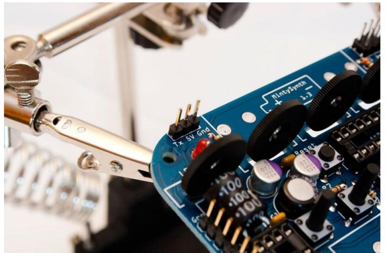
Now install the power switch (it doesn't matter which way, just make sure to hold it vertical and seated as far as it will go while soldering. It doesn't like to stay in the correct position until soldered ;)).
