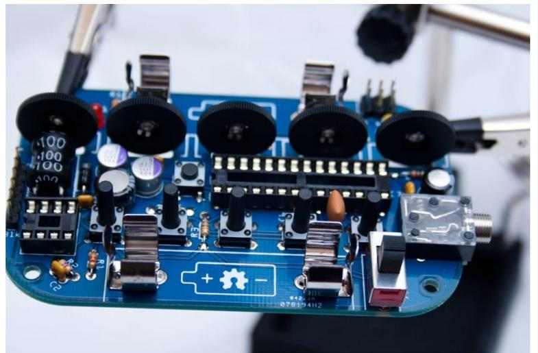
Now we're done soldering, and it's a good time to make sure that you've clipped all leads and pins short on the back, and that none of them extend more than about 1 mm. Also check for small bits of solder or ends of pins that are stuck to the PCB and may cause shorts circuits.
