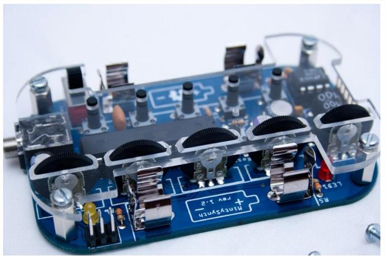
Then reinstall the two remaining screws underneath the PCB on the right side (the side with the audio jack, it's actually on the left in this photo).
