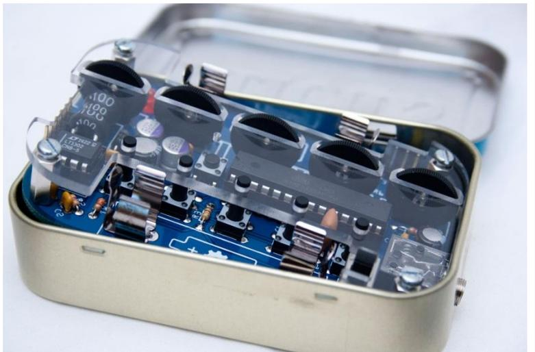
Finally, engage the two screws in the tin into the bottoms of the hex standoffs (they may take a little wiggling), and tighten them. Then screw the small knurled nut onto the outside of the audio jack. Using fingers for this is probably best so you don't scratch the side of the tin.
