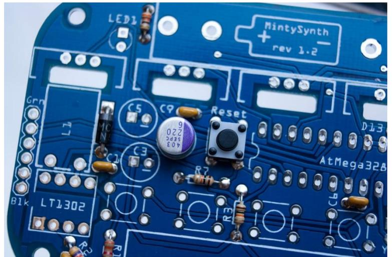
Here you can see the four polarized capacitors installed in the proper orientation.
