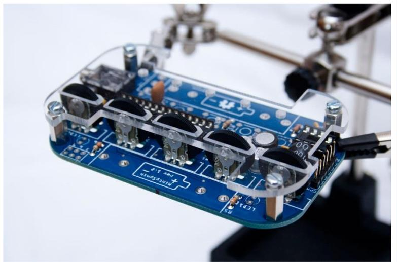
Then you can turn the assembly over and solder all five thumbwheels. Use plenty of solder so that it flows through the holes and flows onto the pads on the top side of the PCB as well. This will ensure a strong mechanical connection. Here you can see we've used enough solder to flow through to the top side.
