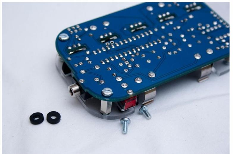
Now tilt the device into the tin, engaging the audio jack in the hole on the side. Then drop the left side down into place. It may take a bit of wiggling, especially if you used a paper punch for the audio jack hole and it is slightly shy of  $\frac{1}{4}$ " in diameter.
