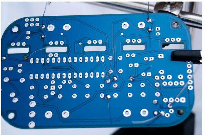
Next we'll add the small yellow ceramic capacitors, C1, C2, C6, C7, and C9. These are all the same, so you don't need to worry about the value. There's also no polarity, so they can go either way. Try to make sure that they are fully seated in the PCB, and sitting vertical. Capacitor C1 is shown here.
