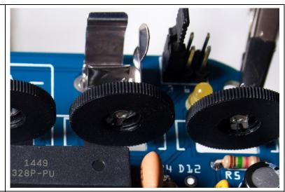
Now we can put the ATmega328 in its socket. You will have to gently bend both rows of pins inward slightly by laying the ATMega on its side on a table and gently folding it over until the row of pins is vertical (then repeat with the other row).
