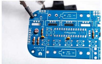
Next is the socket for the ATmega328. The small notch on one end of the socket should point to the left, as an indicator of which way the microcontroller will go later. You can bend the four corner pins outward to hold it in place while you solder. It helps to solder to corner pins first and then checking to make sure the socket is fully seated before committing to soldering the rest.
