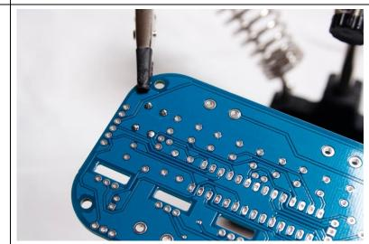
Next you can solder the rest of the resistors in place. R3 and R4 are 150  $\Omega$ , and R5 is 1.5 k $\Omega$ .
