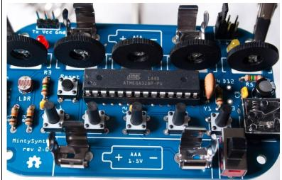
If you'd like you can now put AAA batteries in the device (always noting proper polarity) and turn it on. You should see the LEDs flashing.
