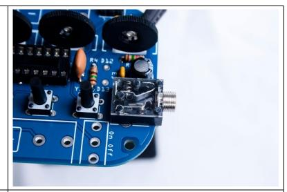
Then install the power switch (it doesn't matter which way). This is another one that can be a little tricky to keep fully seated and vertical while you solder, so take your time and use some means of holding it in place correctly. Be generous with solder here too.
