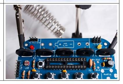
Now we'll add the audio jack as shown. These pins are bigger than on any previous components, so it will take more solder to make a good joint. Use plenty so the jack will be firmly attached to the PCB.
