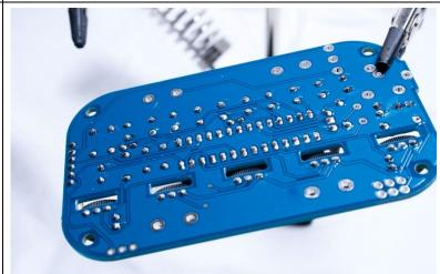
Now add the three headers, with the short ends of the pins in the PCB. These can be a little tricky to hold vertically while you solder, so again use the helping hand where necessary. Solder one or two pins first and check to make sure the header is vertical.
