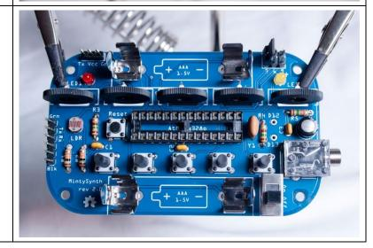
If you'll be using the preinstalled software, put the jumper in place in position 3 as shown. You also have the option of using digital pin 6 or 9 for the audio output if you're using other software. Note: don't forget the jumper, or you won't get any sound. It's easy to forget.
