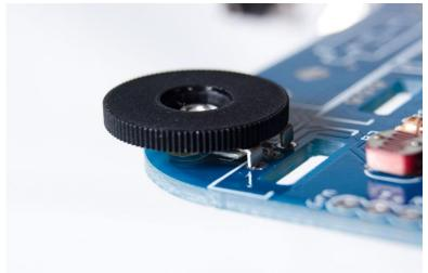
Then gently fold the wheel upward until it is vertical, keeping the pins fully seated in the holes in the PCB as you do this. When you let go the wheel will spring back slightly away from vertical, which is fine.
